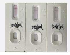
Result zone of the Testing Strip indicates human SARS-CoV-2 N line (T line) and control line (C line). C line must appear to ensure the quality of sample processing. The minimum detectable value for N (SARS-CoV-2) Recombinant Protein is 10 ug/mL.
