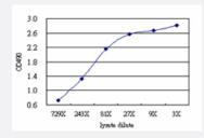
Sandwich ELISA detection sensitivity ranging from approximately 729x to 3x dilution of the HMG20B 293T overexpression lysate (non-denatured).
