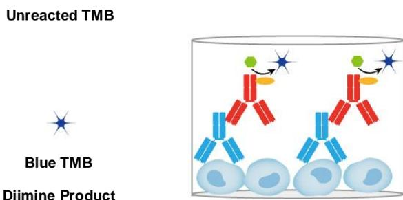
TMB substrate is converted to the blue TMB diimine via the HRP enzyme. Upon addition of acid, the reaction terminates and the wells can be read at 450 nm.
