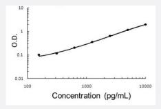
The standard curve is for the purpose of illustration only and should not be used to calculate unknowns. A standard curve should be generated each time the assay is performed.
