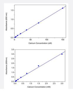
Top: Standard Curve of Calcium Assay Kit (Cat # KA4081) with regular protocol. Calcium dose response was measured on a 96-well black plate with the Calcium Assay Kit (Cat # KA4081). As low as ~ 2.5uM Ca<sup>2+</sup> was detected with 5 minutes incubation time (n=3).
